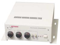
The KAA1000 series is a compact mixer amplifier designed for use in installations requiring paging from a console microphone and from a telephone system. Background music is routed to the output and muted during the announcement. A 2 or 4 tone chime can precede this announcement.
