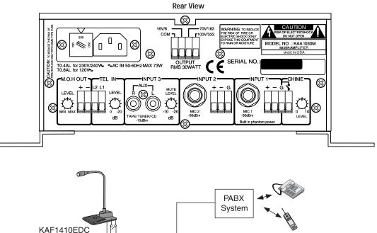
KAF1410EDC PABX Interface +48VDC KAT3233RE Chime 2 3 1 Mixer/Amplifier KAA1030M 8 8 NPUT 30W / 100V OWER ģģ 8
