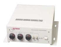
The **KAA1000 series** is a compact mixer amplifier designed for use in installations requiring paging from a console microphone and from a telephone system. Background music is routed to the output and muted during the announcement. A 2 or 4 tone chime can precede this announcement.
